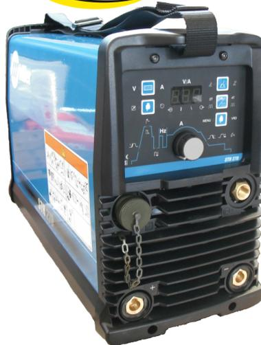
**Remote amperage control** provided through 14-pin receptacle on front of the machine. This permits use of standard remote amperage control devices.
